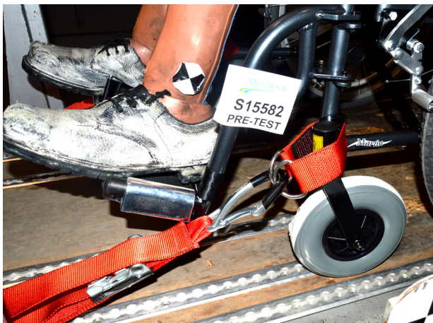
Fitting the Front Restraint
