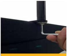
Tighten the two screws with 6mm Allen key **(6)**.
