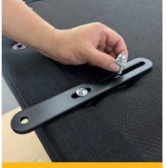
Use two sets of M8 screw (7) and washer (8) to fix one connecting part.
