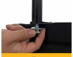
Connect armrest (1) with connecting part using two sets of M10 screw (5) and big washer (6).
